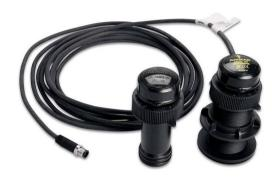
Includes blanking plug to allow active element to be removed for cleaning or maintenance. Skin fitting features a "self seal" flapper valve to minimise water ingress when transducer removed and blanking plug inserted.
